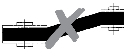
Axial misalignment of sheaves
